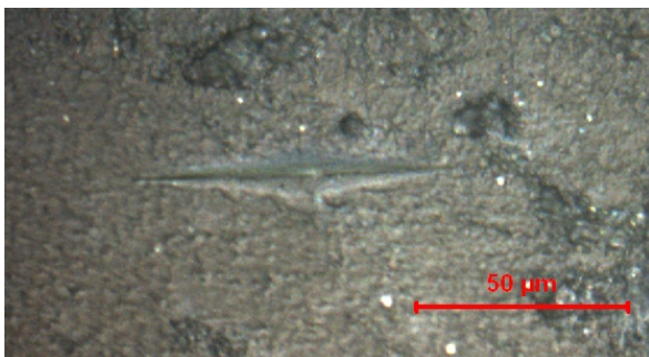
Fig. 4. Representative indentation on cortical bone.
