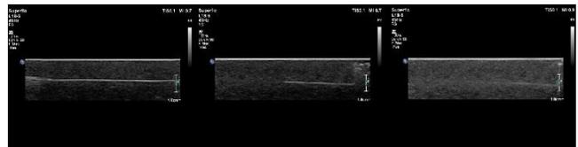
Figure 1: Ultrasound images indicating that capillary channels are seen via ultrasound. The channel was gradually filled with water. Artefacts from the needle used to inject the water is seen in the left part of the imaget.
