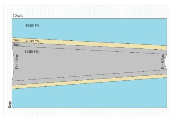
Figure 2: Section of the complex phantom; the first part (grey) in which the micro vessel is placed, the second part simulating the connective tissue (yellow) and the surrounding tissue (blue). Each layer is made of a certain phantom material with properties that are similar to those for the arterial wall.
