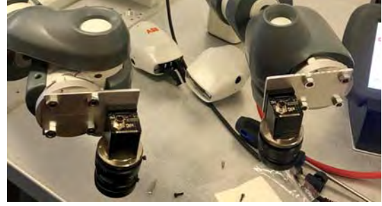
Fig. 5. The prototypes in metal attached to the YuMi robot
