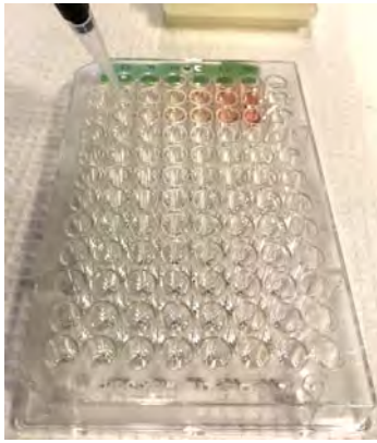
Fig. 3: ELISA plate with wells. Dilution series for HbA in PBS shown at the top.
