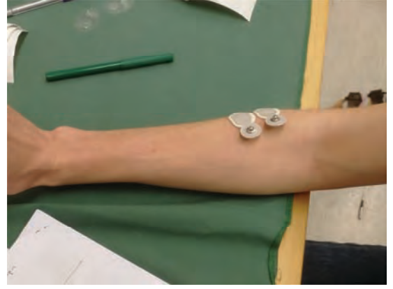
Figure 7. Electrodes placed on the most prominent part of the extensor muscles of the forearm.
