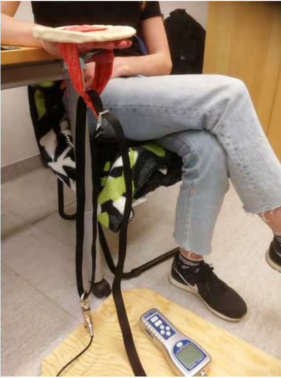
Figure 4. Testing of a preprototype made of salt dough with existing force measuring equipment. An inelastic black band connects the preprototype with load cell.
