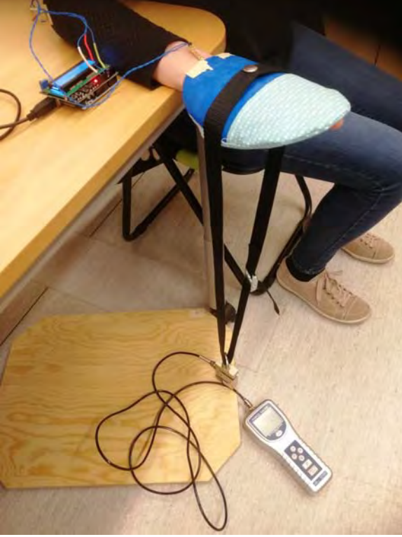
Figure 6. Calibration of the force sensitive resistor by performing resisted wrist extensions with a load cell and dynamometer as reference.
