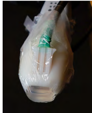
Figure 1. A close-up view of the PA probe used. Here the ultrasonic gel pad is placed in the probe with the plastic foil to keep it in place.
