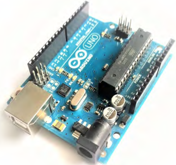
Figure 3. Arduino Uno R3 - microcontroller used to control the iLED 7 surgical light system
