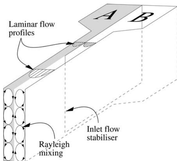
**Fig. 4** Drawing of the test channel. The flow divider was introduced to ensure vertical flow lamination of the two fluids (A and B in the drawing) in the high-aspect-ratio channel. The acoustic standing wave was formed between the channel bottom and the Pyrex lid transverse to the flow
