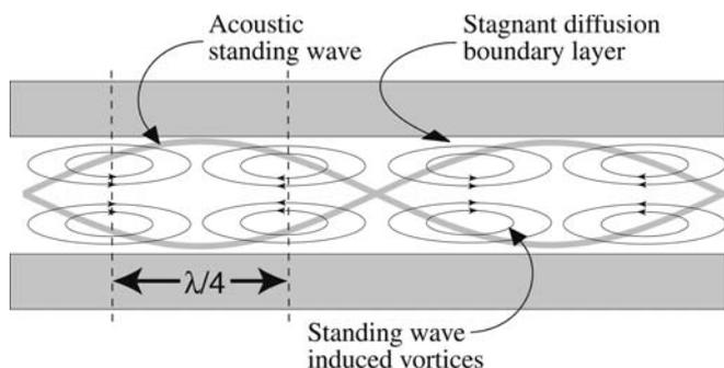
**Fig. 1** Schematic diagram of how an acoustic standing wave field, in a sufficiently narrow channel, induces several vortices spaced  $\lambda/4$  apart
