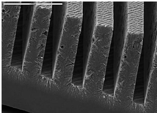
**Fig. 2** Cross view of a high-aspect-ratio parallel-channel enzyme reactor in porous silicon. Each channel is 25  $\mu\text{m}$  wide and 300  $\mu\text{m}$  deep with a 75  $\mu\text{m}$  separating wall in between
