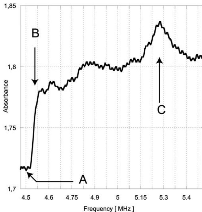
**Fig. 7** Absorbance at 251 nm, measured at the outlet of an enzyme reactor digesting  $0.5 \text{ mmol L}^{-1}$  BAEE at a flow rate of  $16 \mu\text{L min}^{-1}$ : (A) ultrasound power switched off, (B) ultrasound power switched on, (C) Rayleigh flow-induced mixing
