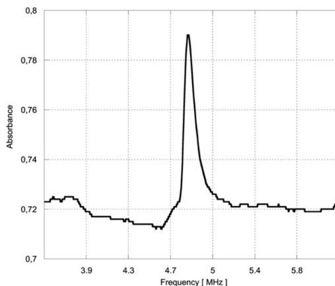
**Fig. 5** Absorbance at 261 nm, measured at the outlet of the test channel, for different frequencies of ultrasonic agitation and a flow of 10  $\mu\text{L min}^{-1}$
