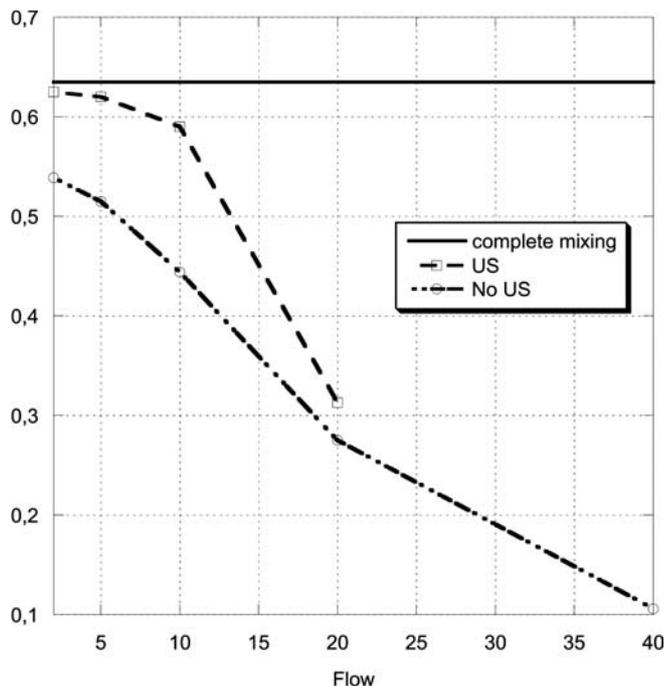
**Fig. 6** Absorbance at 261 nm, as a indication of the efficiency of mixing, measured at the outlet of the test channel for different flow rates, with and without ultrasonic agitation
