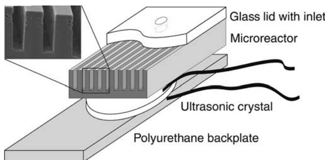
**Fig. 3** Schematic view of the set-up with the enzyme reactor, ultrasonic crystal, and polyurethane back plate
