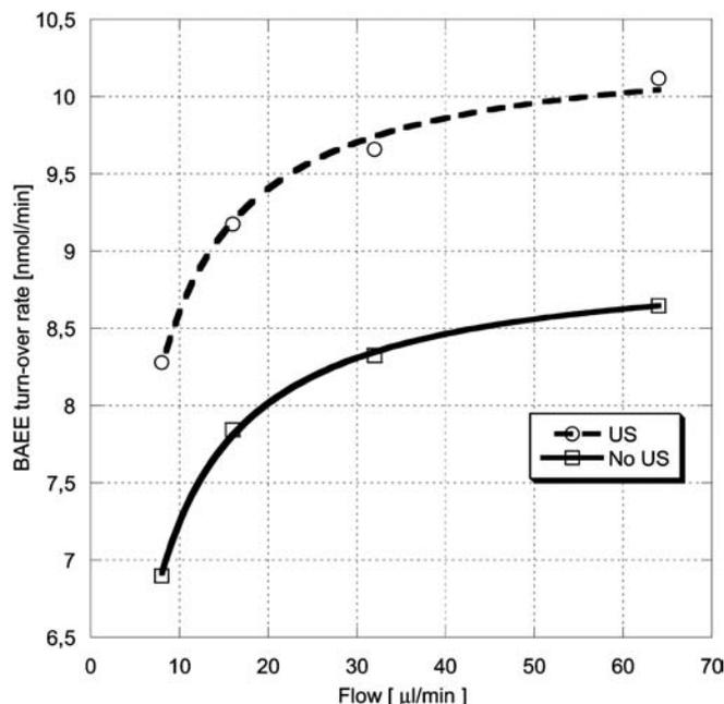
**Fig. 8** Enzymatic turnover in a reactor digesting  $1 \text{ mmol L}^{-1}$  BAEE, at different flow rates, with and without ultrasonic agitation
