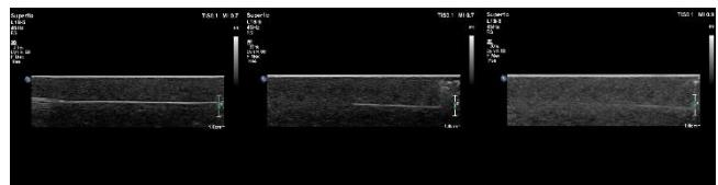
Figure 1: Ultrasound images indicating that capillary channels are seen via ultrasound. The channel was gradually filled with water. Artefacts from the needle used to inject the water is seen in the left part of the image.
