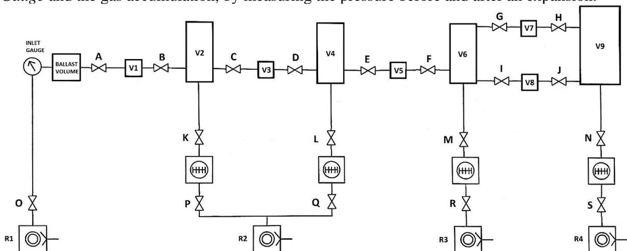
Figure 1: SEA5 at RISE. The gas inlet starts from the left side of the figure through V1, and the finale low pressure is generated at V9.
