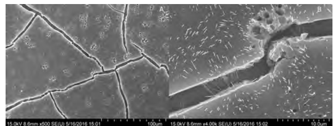
Fig. 10. SEM images showing nanowires on sacrificial layer and PCL, 100 \mu\text{m} scale bar (A), 10 \mu\text{m} scale bar (B).
