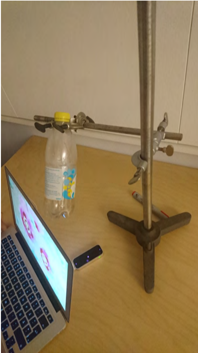
Figure 6. The setup when testing the motion of grabbing the bottle with the whole hand. The Leap Motion Controller is visible.
